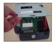
Ensure the UPS battery is connected via the white connector. Use a pen or screw driver to push the dip switch to the side away from the connector (towards the bottom of the unit) to enable the backup battery.
